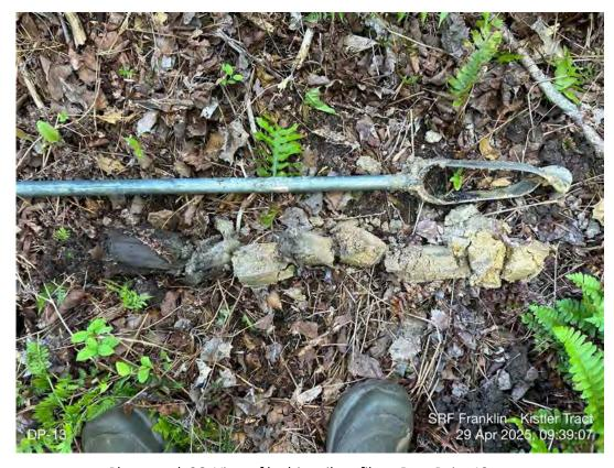
Photograph 26: View of hydric soil profile at Data Point 13.
