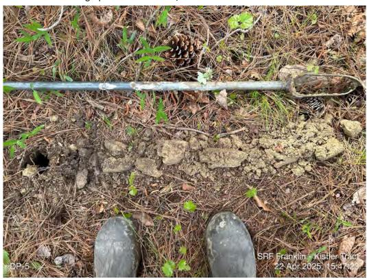
Photograph 10: View of hydric soil profile at Data Point 5.
