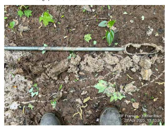
Photograph 8: View of hydric soil profile at Data Point 4.
