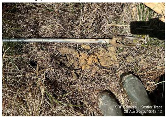
Photograph 22: View of hydric soil profile at Data Point 11.
