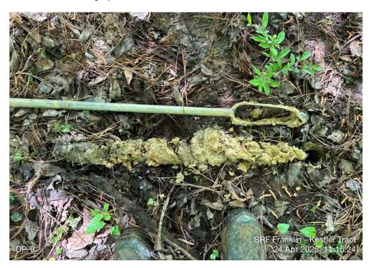
Photograph 18: View of hydric soil profile at Data Point 9.
