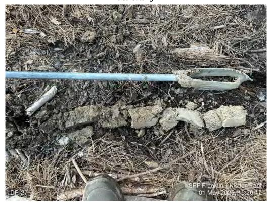
Photograph 53: View of hydric soil profile at Data Point 27.
